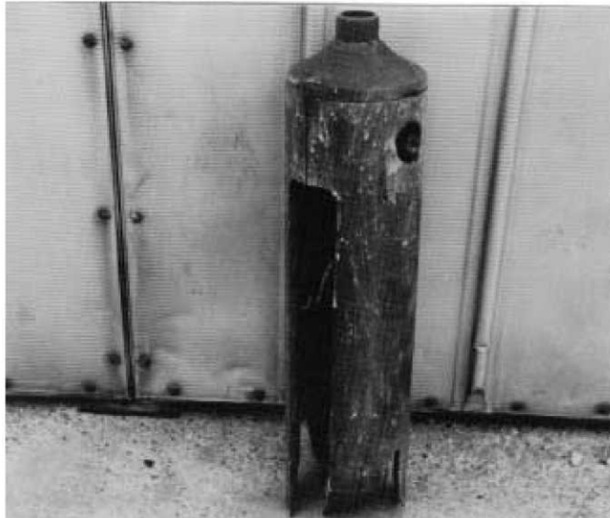
Figure 7-3. Photograph of the McCart split barrel-type auger
